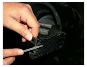
Step 3: File and/or sand down the cut area to make as smooth as possible.
