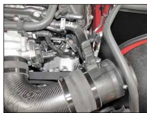
17. Reconnect the mass air sensor electrical connection.
