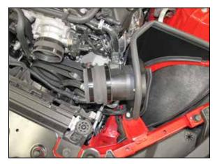
13. Install the provided hump coupler hose (084101) onto the mass air sensor housing and secure with the provided hose clamp.
