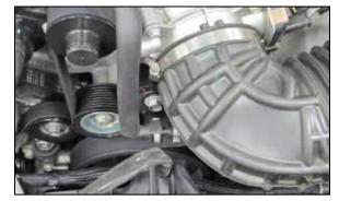
3. Release the quick disconnect fitting and then disconnect the crank case breather vent line.
