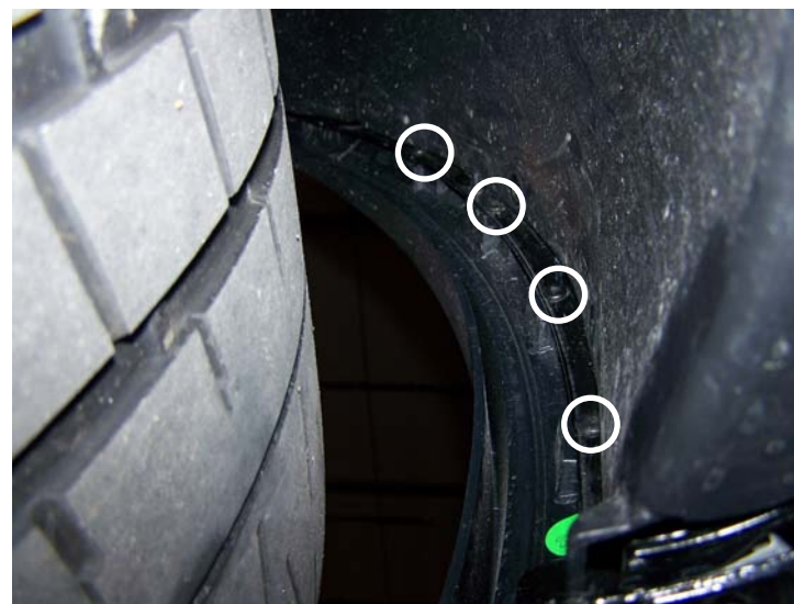
Remove Screws (4 Per Side) From Fender Flare
