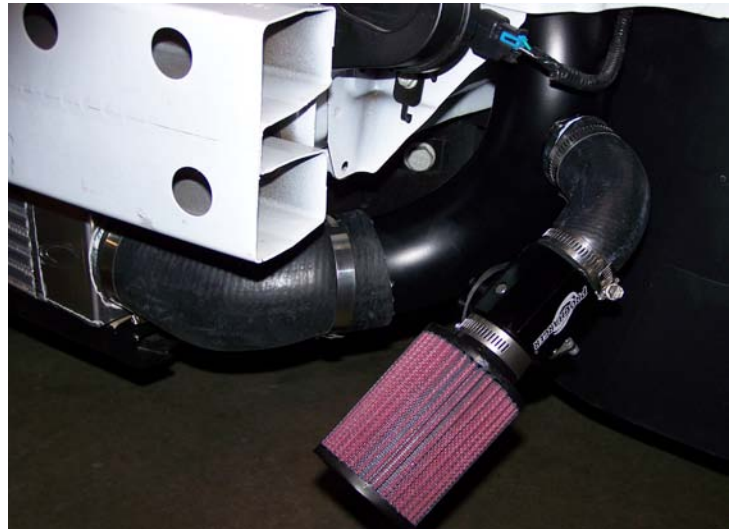
Proflow Surge Valve Installed
