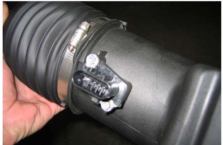
Remove Factory MAF From Intake Tube
