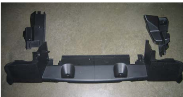
Radiator Shrouding Removed
