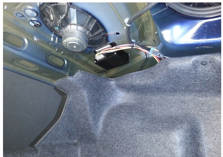
Fuel Pump Booster Installed
