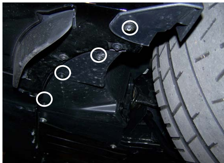
Remove 7mm Screws (4 Per Side) From Bottom Of Inner Fender
