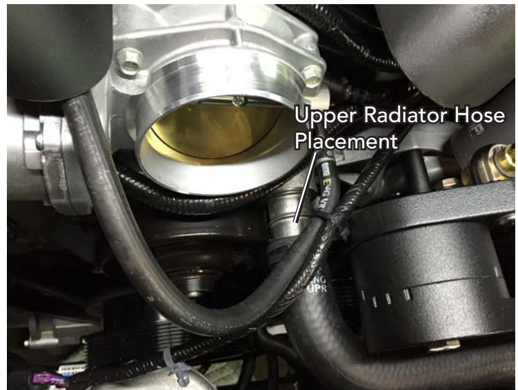
Coolant Hoses Installed
