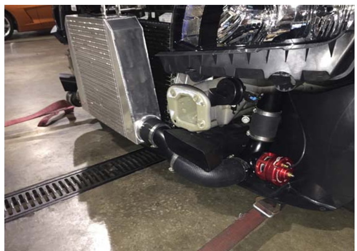
Tubing To Race Intercooler Installed
