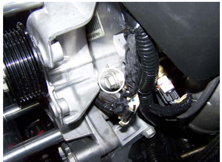
Ground Wire Relocated
