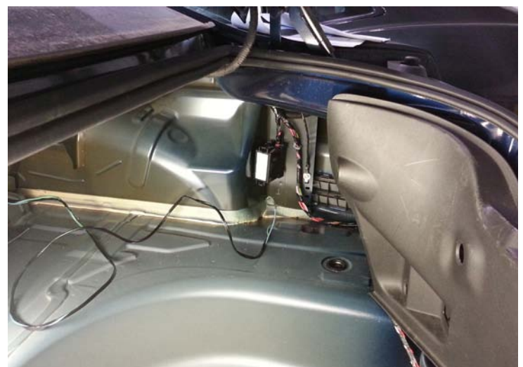
Trigger Wires and Trunk Fusebox
