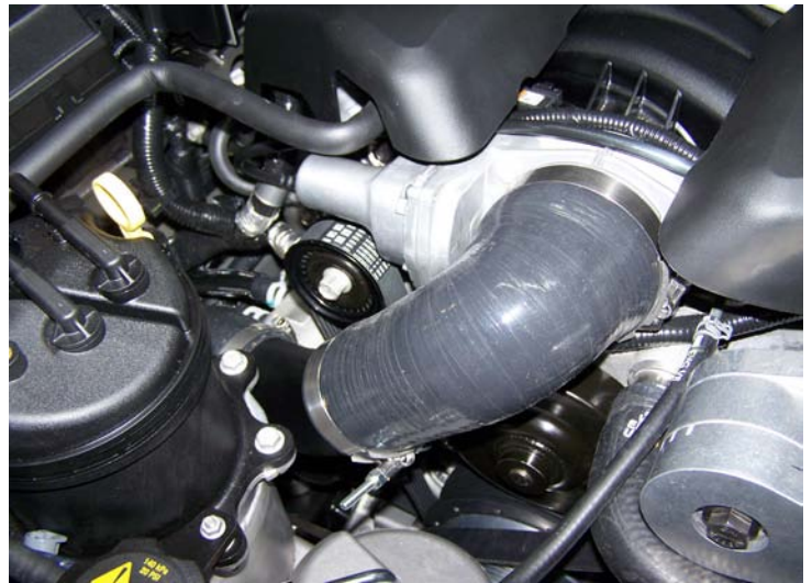
Throttle Body Tube Installed
