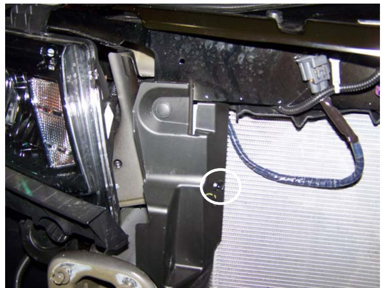
Unclip Ambient Air Temp Sensor
