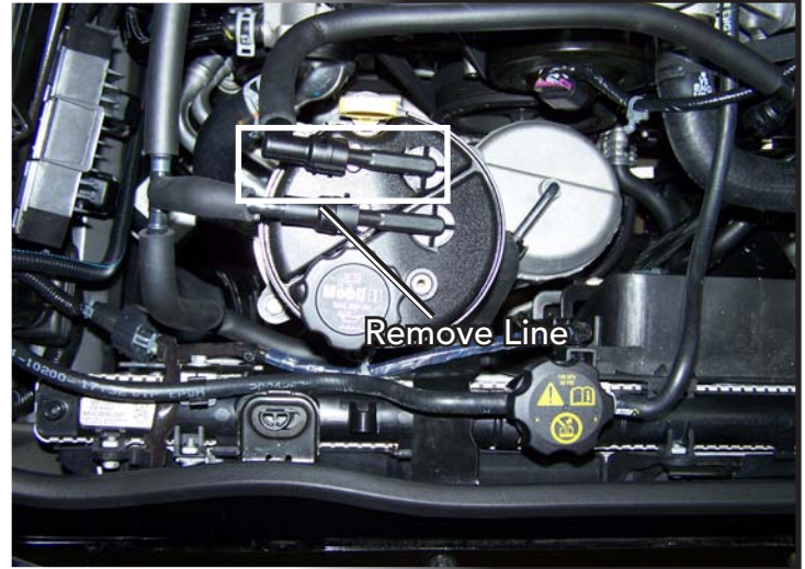
Dry Sump PCV Line
