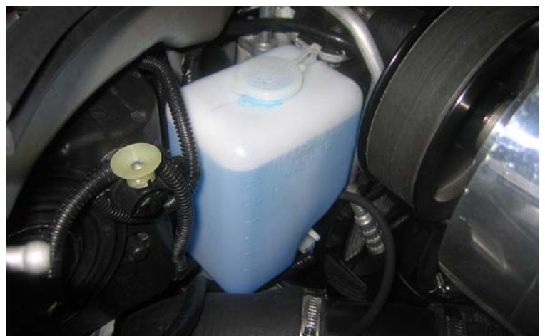
Windshield Washer Reservoir Installed
