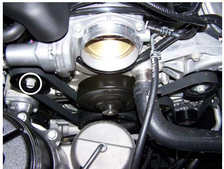
Loosen Tensioner and Remove Belt
