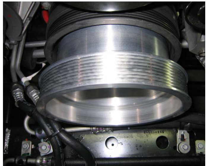
Crank Pulley Installed
