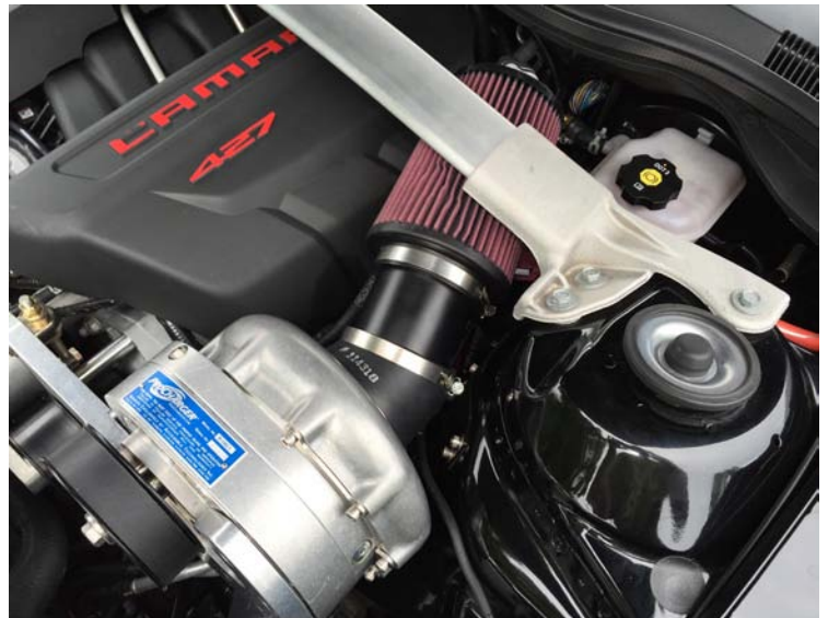
Air Inlet Assembly Installed
