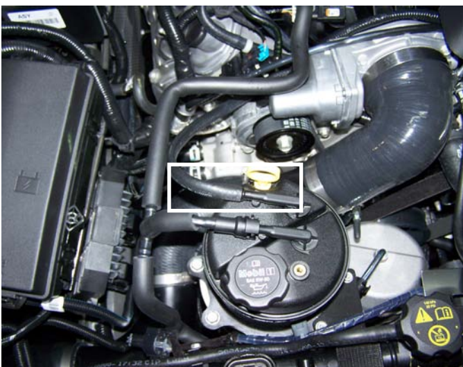
Hose Attached To Dry Sump Tank
