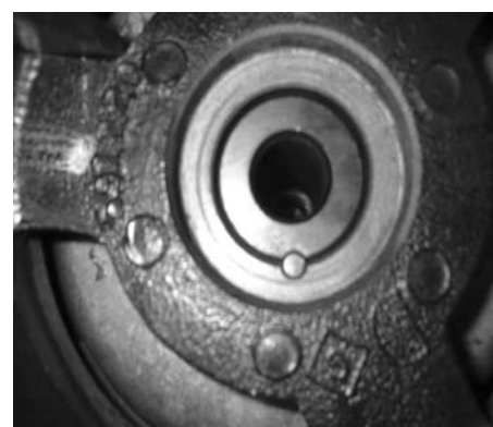
Balancer Pinned to Crankshaft
