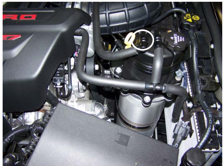
Dry-Sump PCV Line
