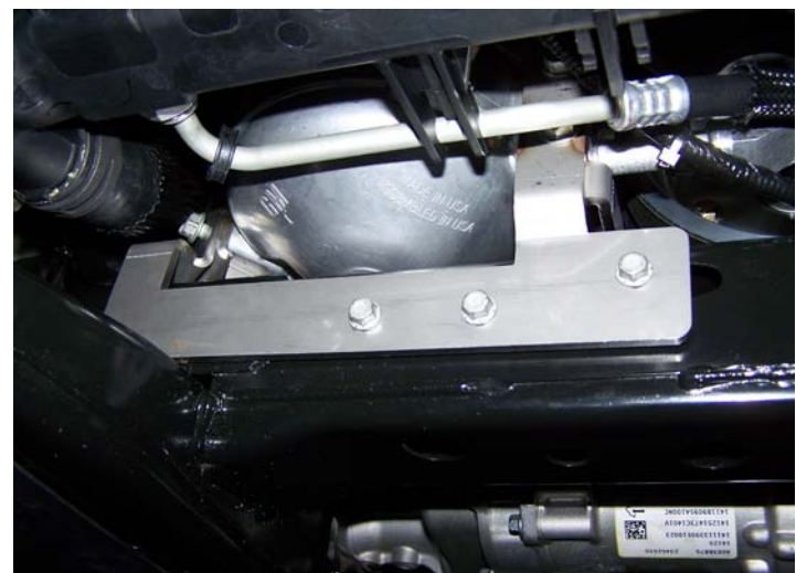
Bottom Dry Sump Bracket Installed
