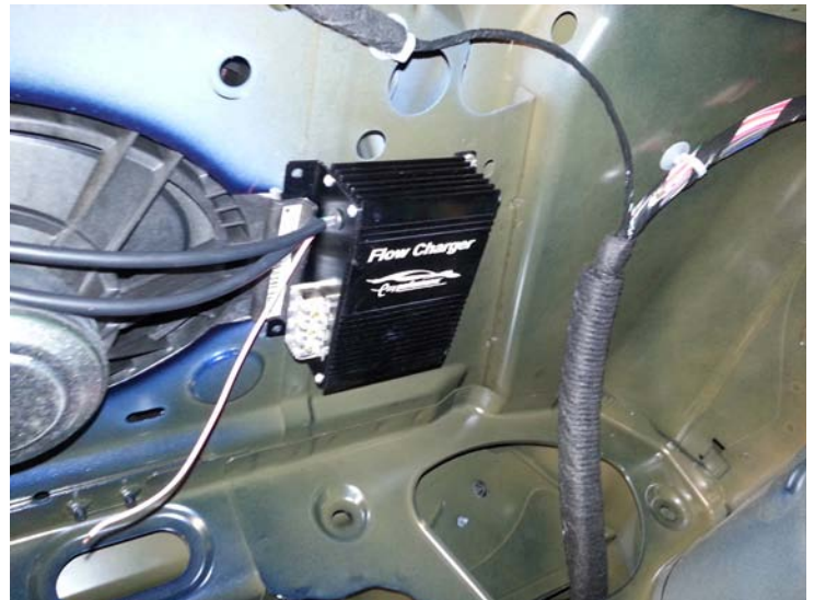
Fuel Pump Booster Mounted
