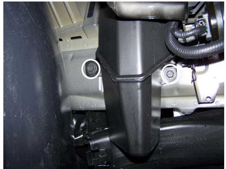
Remove Coolant Reservoir
