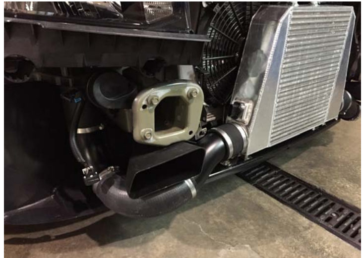
Tubing Out Of Stage 2 Intercooler Installed
