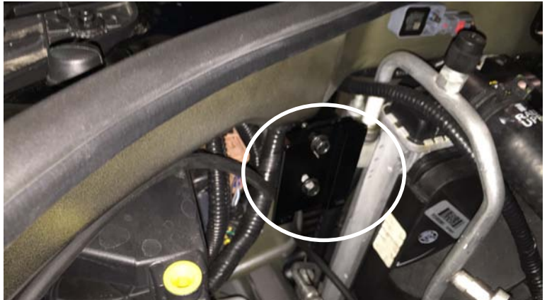
Windshield Washer Reservoir Brackets Mounted
