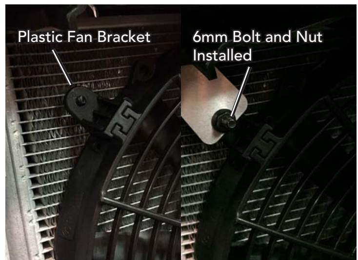
Plastic Fan Bracket / 6mm Bolt &amp; Nut
