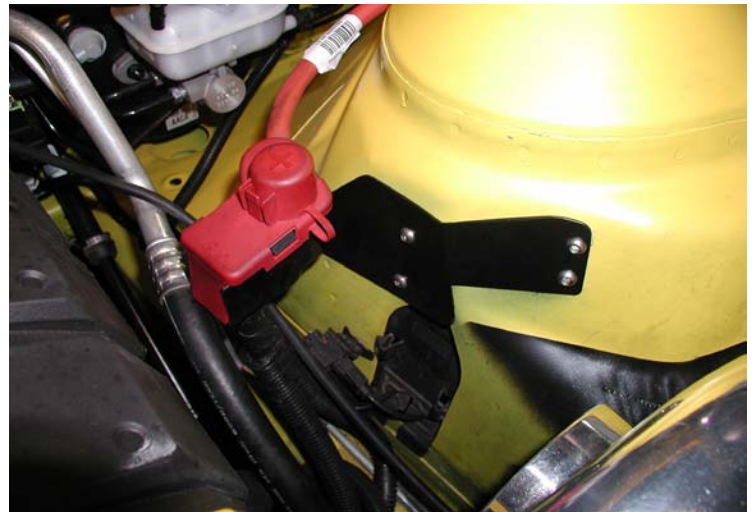
Auxiliary Battery Post Relocation Bracket Installed
