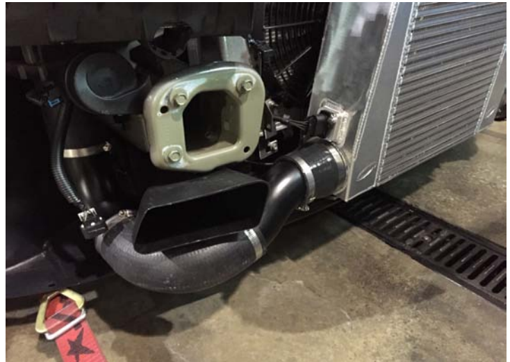
Tubing Out Of Race Intercooler Installed
