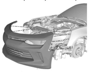
8. Disconnect one electrical connector from driver side before removing bumper entirely.
