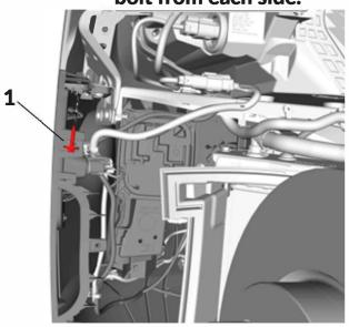
7. Use a small flat bladed tool to depress the lower bumper tabs and pull bumper off slowly.
