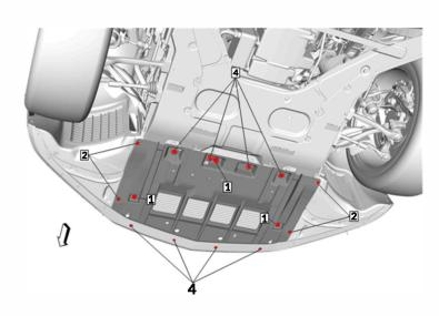
5. Remove 4 bumper bracket bolts from each side.
