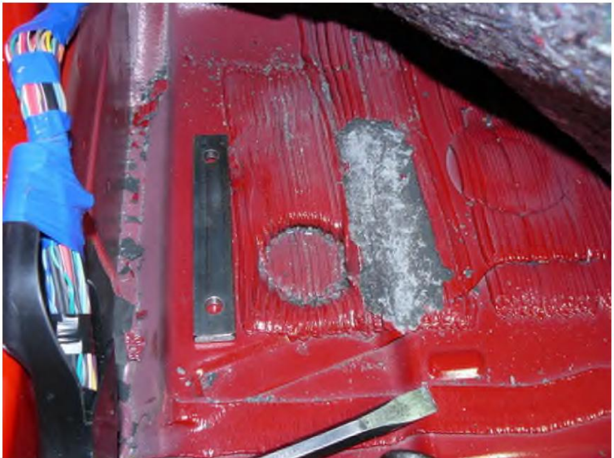
Figure 5. Remove Sealer where main hoop attaches to floor board.
