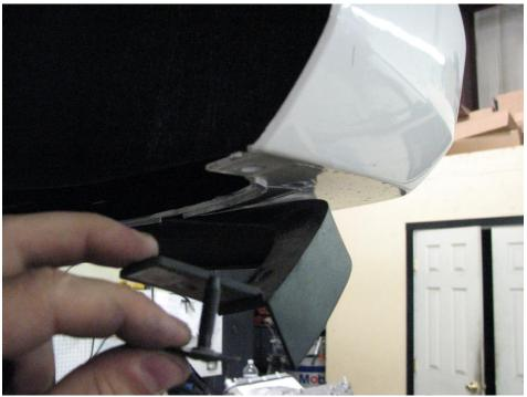
Figure 1: Removal of 2 outermost fasteners
