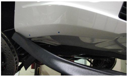
Figure 3: Marking of holes to be drilled
