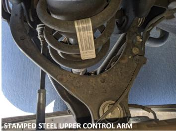
If your vehicle came equipped with the cast steel upper control commonly equipped (but not limited to) to the 07-15 models the proper kit is following:
