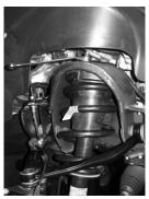
11. Remove the two spring strut assembly lower mounting nuts.
