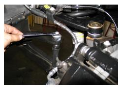
13. Once all the mounts have been un-bolted, hold the spindle assembly while slightly pushing down, dislodging the bottom spring/strut assembly from its lower mounts. Carefully remove the entire spring/strut assembly from its perch, paying extra attention to not damage or over extend brake hoses.
