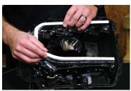
5. Place your new LED Halo on top of the factory optic assembly. We recommend using either double-sided adhesive or epoxy to adhere the halo to the factory optic assembly. Be sure to place whatever adhesive you choose evenly around the halo to ensure secure placement.
