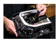
6. Route the wire outside of the headlight, sealing any holes you may create. Reinstall the silver bezel using the original screws. Repeat the process for the other headlight.
