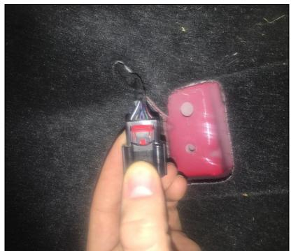
Figure 15 Throttle Pedal Connection
