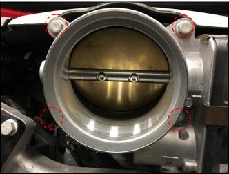
Figure 8 - Throttle Body Removal
