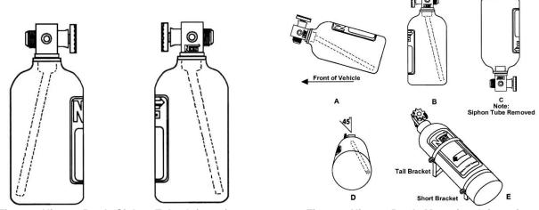
Figure 2 Nitrous Bottle Siphon Tube Orientation
