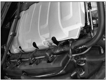
Figure 13 - Fuel Line Routing
