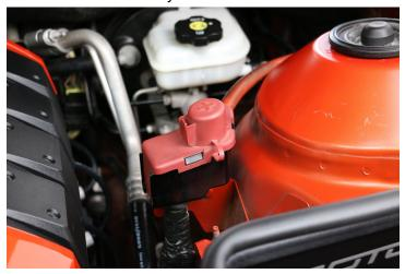
2. Install Wire Loom over Factory Battery Cable. If your Cable has the Hood Cable Attached, then you will need to fit the loom to that point and cut it and use the remainder of the loom for the rest of the cable.
