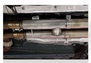
Detail 9: H-pipe and mid pipes installed (factory connect shown)
