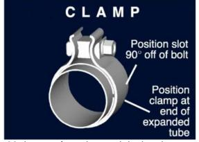
NOTE: Align all clamps so that the center of the clamp bolt is 90 degrees from the notch in the pipe.
