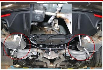
Use a plastic fastener removal tool, or a flat head screw driver to remove the driver and passenger side Christmas tree fasteners (holding the valve actuator wiring harnesses to the brackets) off of the exhaust valves.
