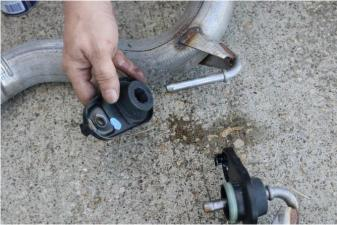
Remove the driver and passenger side hanger grommet assemblies from the axle pipe hangers using grommet pullers or a similar device. Save for Install Step 5.
