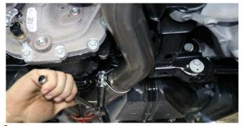
8. Tighten the clamp connecting the passenger muffler inlet pipe to the X-Pipe outlet using a ratchet and 15mm deep socket until muffler assembly is snug on the X-Pipe.
