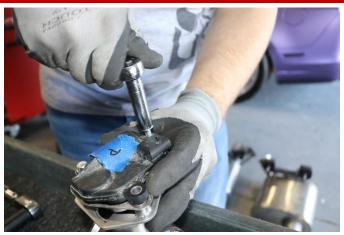
12. Line up the holes on the passenger actuator to the threaded spacers on the valve assembly. NOTE: There will be some resistance from the spring wire form as you rotated the actuator into position. This is normal as it applies pressure on the valve plate to the stops and prevents rattles.
