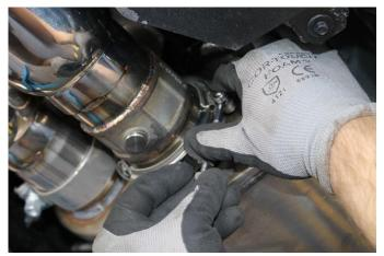
**15.** Mate the v-band flange on the driver valve tip assembly to the flange on the muffler. Align and position the v-band flange so both flanges are fitted within the grooves of the clamp. Reinstall the lock nut and snug the clamp using an 11mm deep socket and 3/8" drive ratchet. The clamp should be positioned with the lock nut towards the inside of the vehicle, the bolt on top and horizontal.
