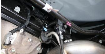
Install the front passenger hanger grommet assembly onto the rear suspension sub-frame and tighten down with the 13mm bolt from Removal Step 4, using a 3/8" ratchet and 13mm socket.
