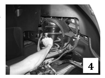
Coil springs may be under tension. Springs under tension store a great amount of energy. Use caution during the following steps to avoid personal injury and/or damage to vehicle. Be careful not to damage or over extend the brake hoses.
