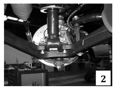
2d. Remove the mount nuts from the end links. Remove the end links completely. This allows the lower control arms to droop further, to ease removal of strut. (**Photo 3**)
