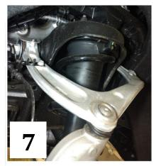
Note it may be necessary to unbolt the upper control arm from the spindle to fit the strut into the mounted position. If this is necessary, remove the upper ball joint nut from the spindle and disconnect the ball joint from the spindle. (Photo 7) Install the Belltech strut following Step 4e. Reinstall the upper ball joint to the spindle and tighten all the fasteners to factory specifications.
