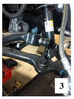
2e. Once all mounts have been un-bolted, hold the spindle assembly while slightly pushing down, dislodging the bottom spring/strut assembly from its bottom mounts dislodging the entire spring/strut assembly from its perch (**Photo 4**)
