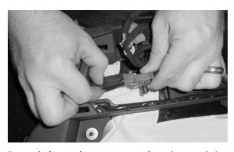
**64. Reattach the rear harness receptacle** to the console base, reconnect the electrical plug, and check the security of the connection.
