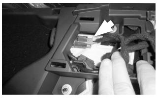
**68. Reconnect the 12v power plug,** and check the security of the connection.
