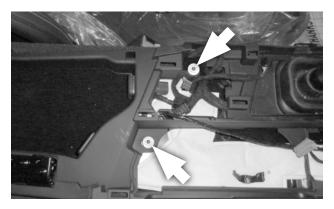
**48. Remove the 2 nuts** at the middle of the console base.
