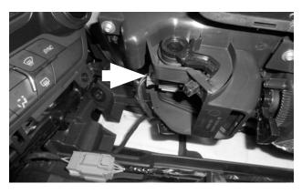
**69. Bring the center console panel back into the vehicle** and tilt it toward the passenger side. Reconnect the cigarette lighter plug, and check the security of the connection.
