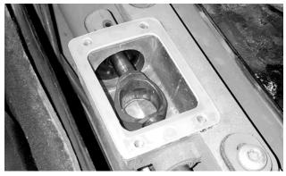
55. Install the new gasket on the mount pad.
