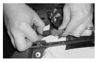
**45.** Release the USB receptacle from the console base, then disconnect the plug from the receptacle by squeezing its locking tabs.
