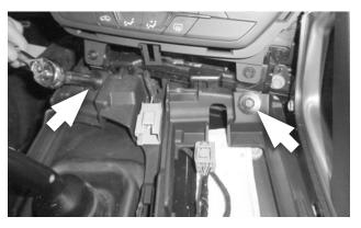
47. Remove the 2 screws at the front of the console base.
