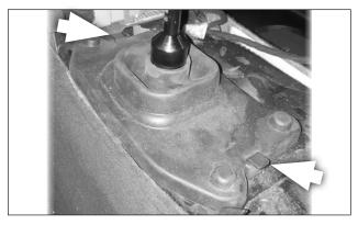
**61. Reinstall the sound insulator,** pushing its slots down over the tabs on the dust boot.
