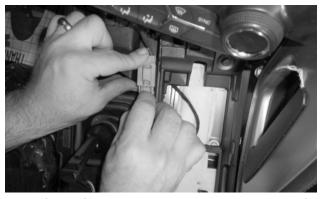
**46.** At the front of the console base, disconnect the plug from the receptacle by squeezing its locking tab, then release the receptacle from the console base.
