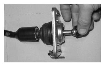
53. Remove the plastic pivot cup from the shift lever.
