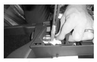
**44. At the rear of the console base,** disconnect the 12v receptacle plug by gently squeezing its sides with pliers while pulling the plug out of its receptacle.
