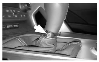
74. Place the knob on the shift lever, making sure that its locking grooves align with pins inside the chrome ring on the leather boot. Apply medium-strength thread locker to the 6mm screw, and secure the knob to the lever at the larger (bottom) screw hole.
