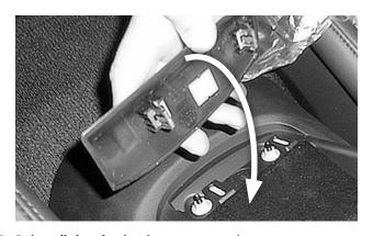
$\textbf{67. Reinstall the plastic trim cover} \ \text{over the rear nuts}.$
