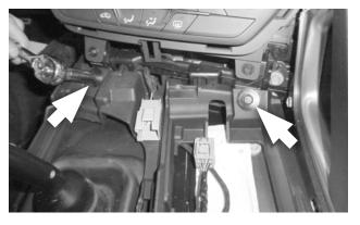
**66.** Hand-start the **2** screws at the front of the console base, then tighten the **2** screws and **4** nuts.
