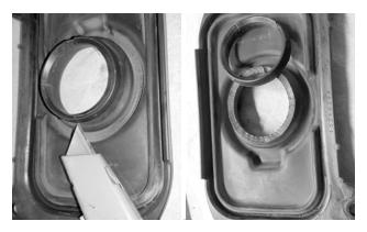
**59.** Use a sharp, new blade to cut the hard plastic edge off the bottom of the rubber dust boot, to allow the boot to fit around the shifter base.
