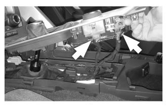
**70.** Reconnect the parking brake and Mode Select plugs, and check the security of the connections.
