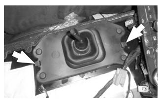
**50.** Release the sound insulation from its **2** tabs, lift it over the shift lever, and set it aside.
