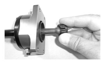
**54. Grease the pivot ball** at the bottom of the **Hurst shifter's** lever. Then snap the stock pivot cup onto the pivot ball.
