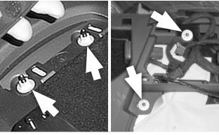
65. Hand-start the 2 nuts at the rear and the 2 nuts at the middle of the console base.
