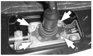
**52. Put the shifter in Neutral.** Then remove the 4 mount bolts and the shifter assembly, and remove any gasket material from the mount pad.
