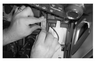
**63.** Reattach the front harness receptacle to the console base, reconnect the electrical plug, and check the security of the connection
