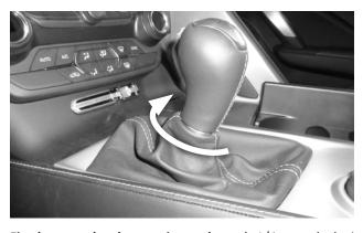
**75.** Firmly grasp the chrome ring and turn it 1/4-turn clockwise to lock it into place on the knob.
