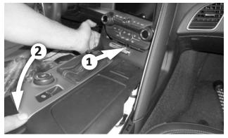
**71.** Starting at the front and working back, reinstall the console panel, ensuring that it is securely snapped into place on all four sides.
