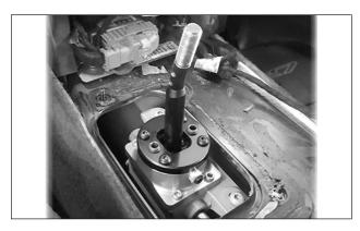
**56. Orient the shifter with the lever's bend to the rear,** and place it on the shift box, inserting the pivot cup into the shift linkage. Apply medium-strength thread locker to the 4 screws, and use them to secure the shifter to the shift box.
