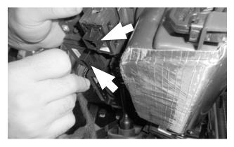
**42.** Carefully tilt the console panel forward to view the 2 rear electrical plugs. Disconnect the Mode Select and parking brake plugs by squeezing their locking tabs.
