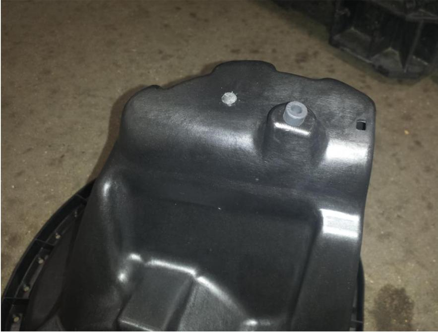
4. Insert the dirty air inlet (1315-9F763-A) into the air box (131550-9A612).
