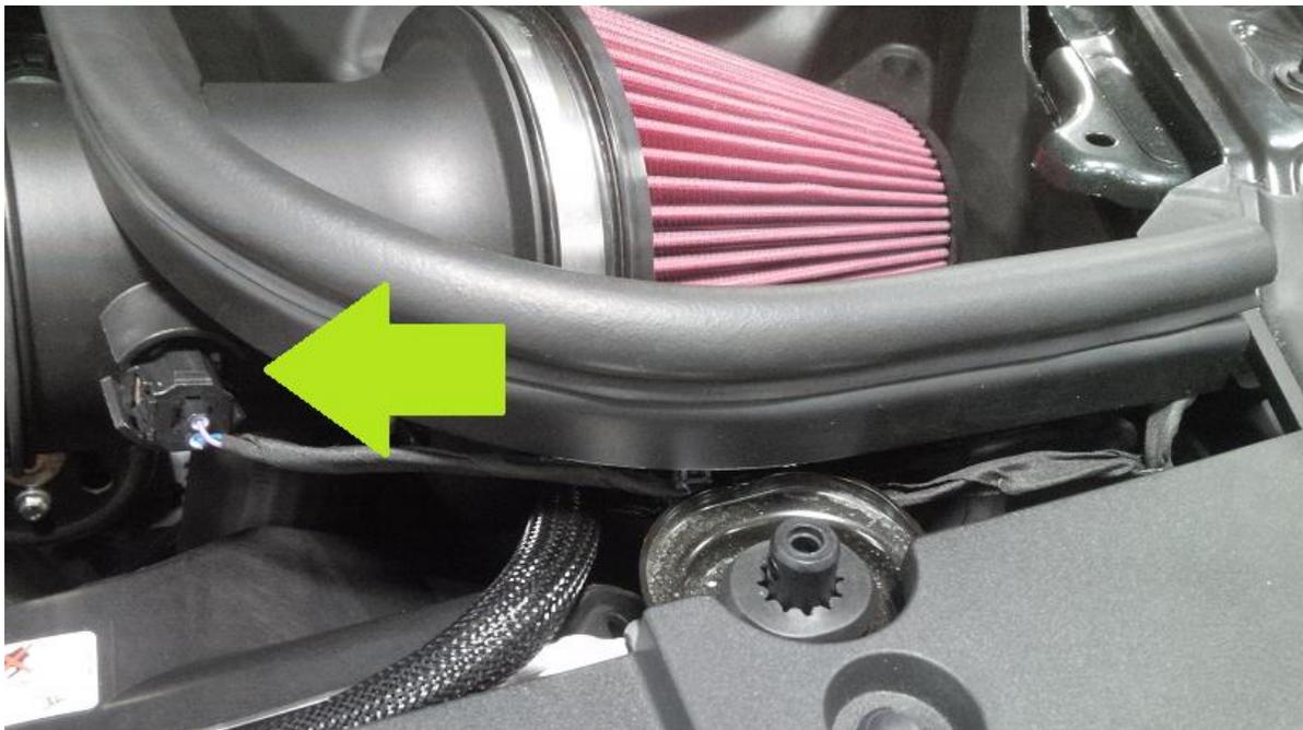
15. Install the clean air tube coupler onto the turbo inlet (Part Number 131523-SILCP-AA) and tighten clamp (Part Number 5340). Use clamp (Part Number 5348) to fasten the clean air tube to the coupler. Lastly tighten the clamp from the clean air tube to the air filter tube (Part Number R07130028-13-AA).
