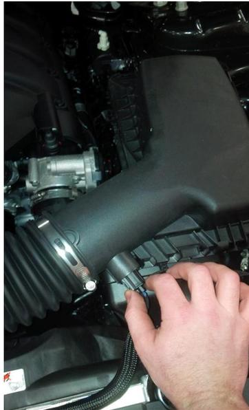
4. Loosen the clamp at the air box from the intake tube.
