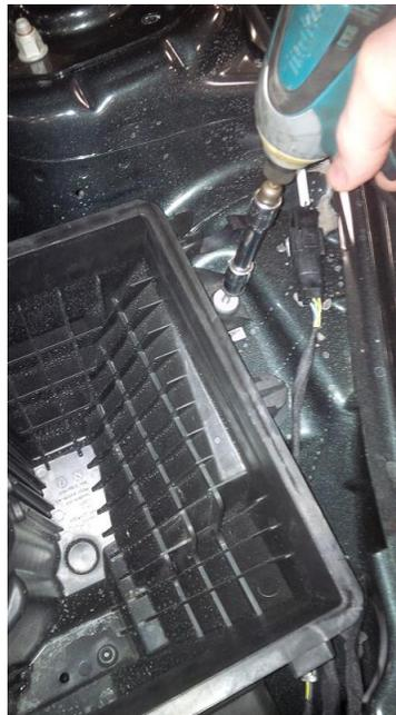
8. Remove the air box tray and dirty air inlet from the car.
