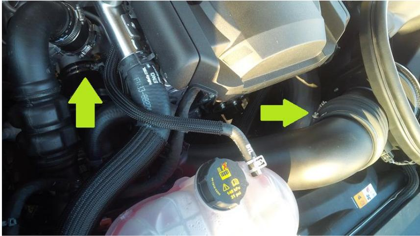
16. Install the PCV tube with the quick connect (make sure it's fully seated), followed by the recirculation valve hose with the constant tension clamp.
