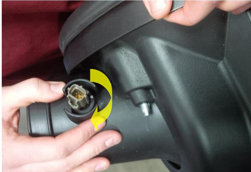
14. Connect the temperature sensor connector.
