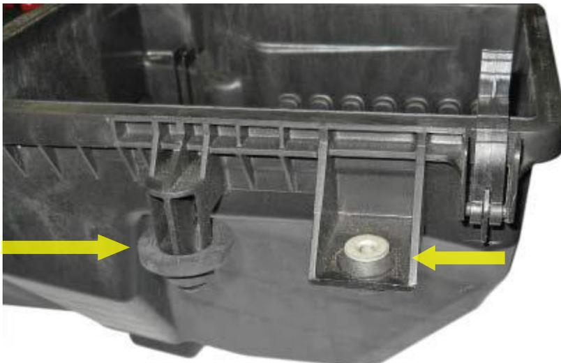
14. Remove the rubber isolator from the bottom of the stock air box tray and retain for later use.
