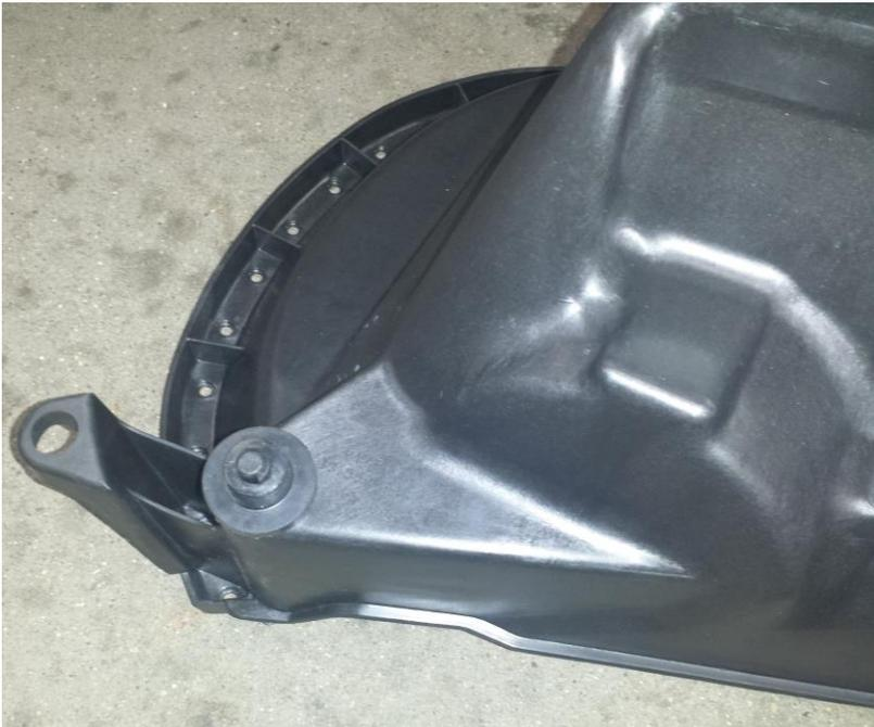
3. Install the rubber isolator into the bottom of the air box (131550-9A612)
