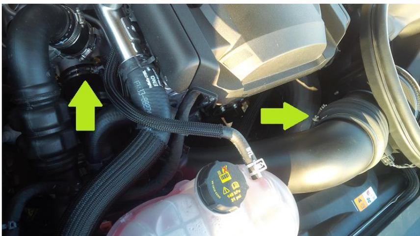
10. Remove the Air Temp sensor from the factory air box by twisting counter clockwise and re-install into the Roush filter tube (Part Number 131523-12B579) by twisting clockwise.
