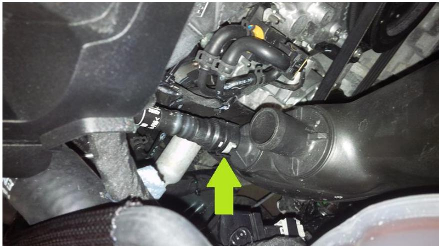
12. Remove the clamp on the turbo inlet end of the clean air tube. Once the clamp is off you can remove the clean air tube and air box from the car.
