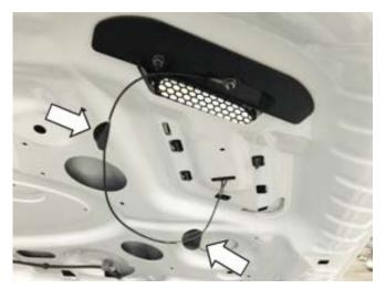
3. Remove two (2) 9 mm nuts, release the retaining clips and remove each factory heat extractor.
