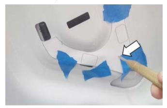
Drill each hole with a 1/4" bit. After the holes are drilled, apply commercially available clear coat (Motorcraft Part Number: PM-19500-6000) to the exposed metal so that it does not corrode.
