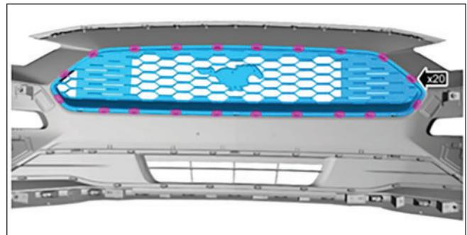
2. Once the ROUSH upper grille is clipped in, reinstall the front bumper cover reinforcement panel by clipping the panel into the six (6) locations on the front bumper cover.
