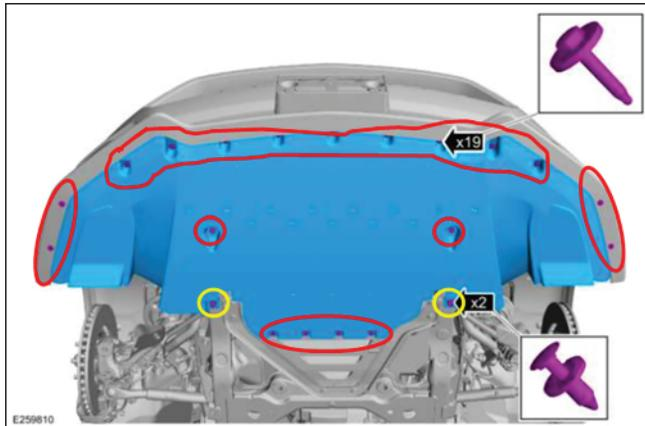
4. Remove the eight (8) radiator close out panel clips. Remove the close out panel.
