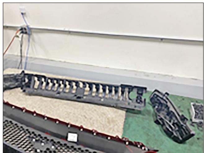
4. Remove the stock upper radiator grille by releasing the twenty (20) tabs that mate with the front bumper cover panel.
