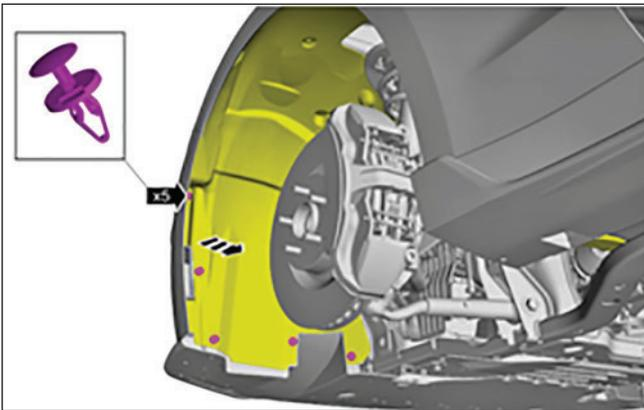
5. Position the close out panel to the vehicle. Reinstall the eight (8) radiator close out panel clips.
