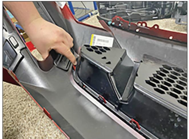
5. Once the clips are released, pull to remove the original grille from the front bumper cover panel.
