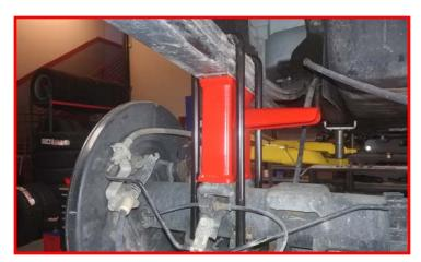
Install the provided shocks using the factory hardware. Do not tighten at this time.
