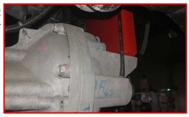
Re-connect the electrical connector on the differential actuator. Make sure to push in the safety lock. Zip tie the harness to the locating holes on the differential housing at the first and second mounts. Leave the one closest to the drive side undone.
