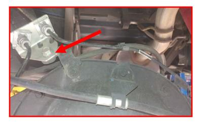
Remove the brake line bracket from the axle and discard. Remove the parking brake from the axle.
