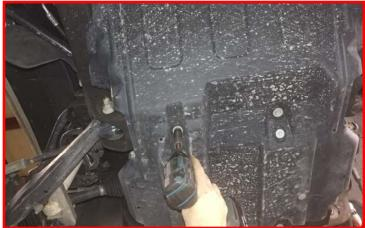
Remove the factory rear cross member from the frame. (2wd: Loosen but removal is not necessary)
