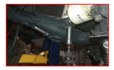
Remove the strut from the vehicle.
