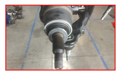
Install the completed ReadyLIFT knuckle assembly to the lower ball joint using the factory hardware while guiding the CV axle through the hub. Install the upper ball joint to the knuckle using the factory hardware if using the factory control arm and provided hardware if using the ReadyLIFT control arm. Torque the lower ball joint nut to 110 ft-lbs, and upper ball joint nut to 85 ft-lbs.
