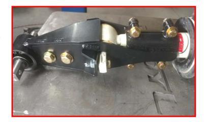
Locate the ReadyLIFT tapered strut shim.
