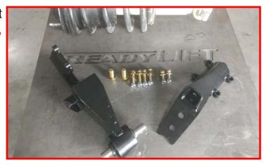
Install the ReadyLIFT clamshell mount around the lower strut body. Make sure to mount the clamshell to the strut with the inside angle towards the frame side of the strut.
