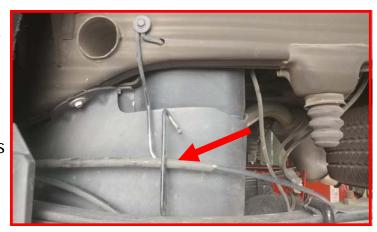
Remove the brake line bracket at the shown point.
