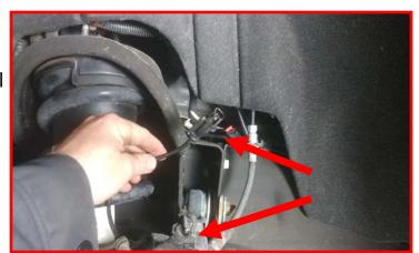
Remove the brake line bracket at the control arm.
