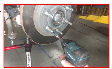
Remove the axle nut cover if installed. Remove the axle nut.
