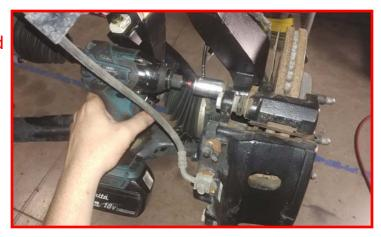
Install the ReadyLIFT brake line bracket to the frame rail using the factory hardware. Hand tighten only as this is a self tapped hole and can strip easily. Gently pull down on the metal line and install the bracket to the ReadyLIFT bracket using the provided 5/16" x .75" bolts, washers and locking nuts. Torque to 5 ft-lbs.
