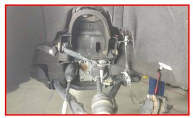
Remove the CV axle from the differential.
