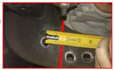
Use a suitable cutting tool, cut along the previously made marks. Sand the rough edges of the frame and paint the exposed metal using a quality rust preventative paint.
