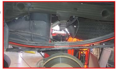
Install the ReadyLIFT block making sure the tapered end goes to the front of the vehicle. Raise the axle while lining up the center pins on the axle and block. Install the provided u-bolts. Do not fully tighten at this time. Repeat for the other side of the vehicle.
