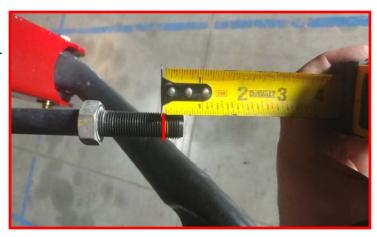
Hold the outer tie rod end in a vice. Measure from the end 1/2" and make a mark. Use a suitable cutting tool and cut off the end. Sand any burs off the end. Install onto the already cut inner tie rod end.
