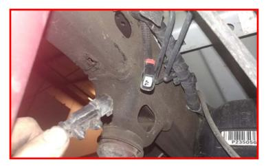
The passenger ABS harness is clipped into the rear cross member and frame rail. Remove the harness from the frame.
