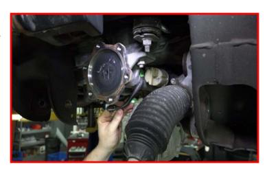
Remove the differential hardware and carefully lower the differential out of the vehicle. Set aside. Use of a helper will aid in the removal of the differential.
