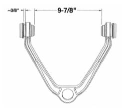
f) For **2007 up** vehicles the distance between the two inner faces of the bushings should be 9. Make sure the bushings are centered in the arm.
