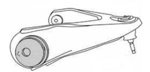
e) For 1999-2006 vehicles the distance between the two inner faces of the bushings should be 9 7/8". Make sure the bushings are centered in the arm.
