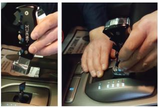
4. Install assembled shifter handle (1).
