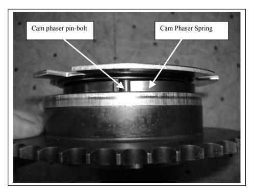
**Step 4:** Using a soft cloth to protect the cam gear, lock just the gear portion of the cam phaser in a vise. Do not over tighten the vise, use just enough force to secure the gear. Position the cam phaser in the vise with the pin-bolt at the 2-3 o'clock position, looking at it from the cam side. Take note that the first bolt located clockwise from this pin-bolt will not be removed. We will be using that bolt to pivot the cam phaser cover out of the way.
