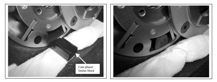
**Step 8:** Rotate the cover plate back over the control chambers and reinstall the safety bolt. Reinstall the cam phaser bolts, making sure to install the pin-bolt back into the correct position. Remember to torque the bolts to 85 in. lbs.
