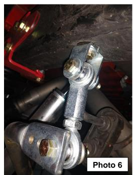
\*\*The end links are adjustable; adjust the end links to get the sway bar as parallel with the ground. This is easily achieved once the vehicle is flat on the ground. \*\*
