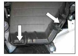
6. Unlatch the upper air box clips and remove the upper air box and intake tube assembly.
