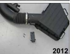
17. Remove the two screws that secure the mass air sensor into the factory intake tube. **NOTE: Vehicle's MAF sensor may vary among**
