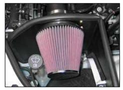
23. Install the K&N<sup>®</sup> air filter and secure with the provided hose clamp.
