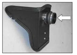
14. Install the provided silicone hose (5-576) onto the filter adapter as shown and secure with the provided hose clamp. model years, reference appropriate image above.
