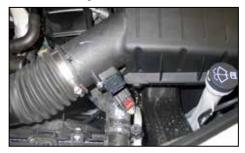
3. Slide the red locking tab back and then disconnect the mass air sensor electrical connection.
