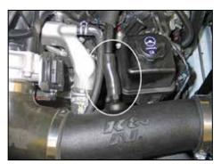
22. Remove the 90° vent hose from the crank case vent tube. Install the provided silicone vent hose and install it onto the fitting installed into the K&N<sup>®</sup> intake tube. Trim the vent hose for proper fit.
