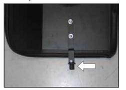
12. Install the provided inserted nut onto the heat shield mounting bracket and secure with the provided hardware.
