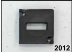
16. Install the provided gasket onto the mass air sensor adapter.
