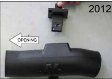
19. Install the mass air sensor assembly into the  $K\&N^{\mbox{\ensuremath{\mathbb{S}}}}$  intake tube as shown and secure with the provided hardware.
