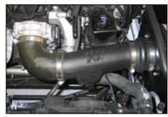
21. Install the provided silicone hose (08629) onto the K&N<sup>®</sup> intake tube as shown. Install the K&N<sup>®</sup> intake tube assembly onto the throttle body and hump hose attached to the filter adapter. Adjust the intake tube in the hoses for proper fit, once proper fit is achieved secure the tube with the provided hose clamps.
