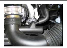
4. Disconnect the crank case vent hose from stock intake tube.
