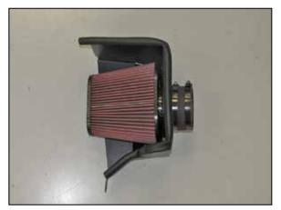
17. Set the air filter into the heat shield and then install the provided coupling hose (08761) onto the filter and secure with the provided hose clamp.
