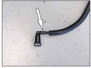
29. On vehicles equipped with a "Wet Sump" oiling system, separate the nylon crank case vent hose from the 90° quick disconnect fitting.
