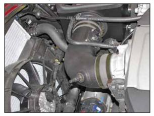
25. Install the K&N<sup>®</sup> intake tube assembly into the air filter coupling hose and then into the coupling hose at the throttle body. Adjust the tube and filter for best fit and then secure with the provided hose clamps.
