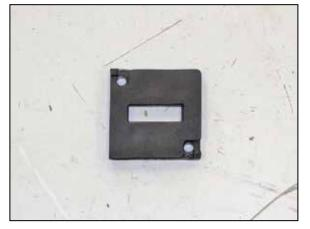
21. Install the provided gasket onto the K&N<sup>®</sup> mass air sensor adapter as shown.
