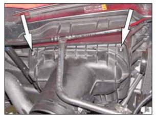
7. Loosen the two TORX fasteners securing
