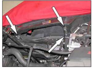
14. Install the three provided rubber mounted studs onto the heat shield mounting location as shown.
