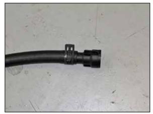
27. On vehicles that are equipped with a "Dry Sump" oiling system, assemble the provided crank case vent hose (08635) and quick disconnect fitting and clamp as shown.
