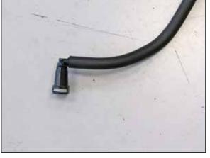
30. Cut the provided crank case vent hose to a length of 15" and install onto the factory 90° quick disconnect fitting.
