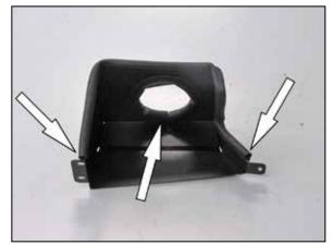
16. Install the 16" section into the hole of the heat shield and install the 27" section around the perimeter of the heat shield as shown. NOTE: Use the provided super glue on the edge trim to hold down the ends next to the inner
