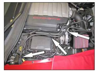
28. On vehicles that are equipped with a "Dry Sump" oiling system, install the crank case vent hose assembly onto the oil tank and then route it through the factory retaining clips and then connect the open end to the 90° fitting installed into the K&N<sup>®</sup> intake tube.
