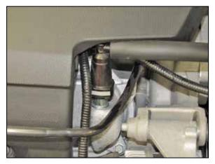
4b. On vehicles equipped with a "Wet Sump" oiling system, disconnect the crank case vent hose from the passenger side valve cover port and remove the hose from the vehicle.
