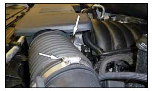
4. Loosen the hose clamps that secures the intake plenum to the air filter housing and to the throttle body. Disconnect the plenum connections at the air filter housing and then rotate the plenum counter clockwise to disengage the keyed mount and separate it from the throttle body. **NOTE: The wiring harness anchored to the intake plenum will need to be detached before removing the plenum from the vehicle.**  release arm to the hood latch and then remove the arm.
