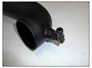
20.Install the provided 90° quick connect fitting into the K&N<sup>®</sup> intake tube as shown. **NOTE: Plastic NPT fittings are easy to cross thread. Install the vent fitting "hand" tight, then turn it two complete turns with a wrench.**
