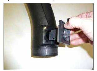
22. Install the mass air sensor into the K&N<sup>®</sup> intake tube and secure with the provided hardware.
