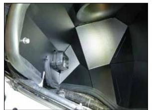
14. Install the heat shield assembly into the vehicle so the mounting grommet slides into the factory
