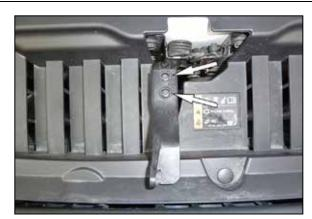
5. Remove the two bolts that secure the hood
