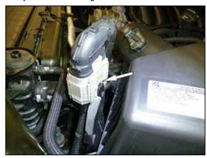
8. Using a small 90° pick or similar tool, release the locking tab that secures the wiring harness bulk connector to the air filter housing and then unhook the connector from the housing.
