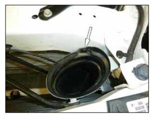
7. Remove the plastic retaining clip that secures the fresh air intake duct to the core support, then pull the duct forward to disengage it from the factory air filter housing.
