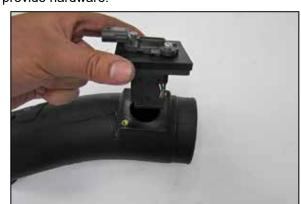
20. Install the mass air sensor assembly into the K&N® intake tube in the direction shown and secure with the provided hardware.
