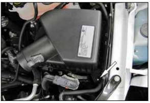
9. Remove the nut that secures the air filter housing assembly to the vehicle. Remove the air filter housing assembly from the vehicle.
