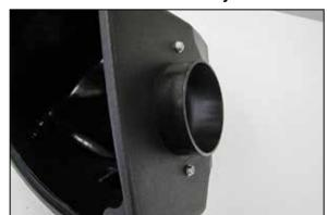
10. Install the provided radius filter adapter into the K&N® air filter housing and secure with the provided hardware.
