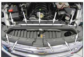
6. Release the ten plastic locking pins holding the upper radiator valence and then remove the valence from the vehicle.
