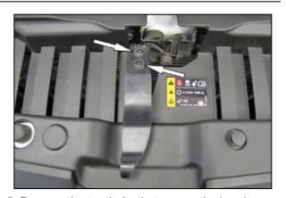
5. Remove the two bolts that secure the hood release arm to the hood latch and then remove the release arm.
