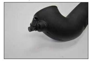
21. Install the  $90^{\circ}$  quick disconnect vent fitting into the K&N® intake tube as shown.
