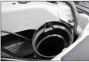
15. Push the factory fresh air intake duct into the K&N® air filter housing and then reinstall the plastic clip to secure it into position.
