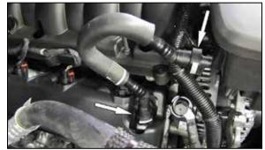
3. Depress the locking tabs and then disconnect the crank case vent line from the intake plenum and valve cover vent port.
