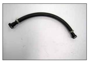
22. Assemble the crank case vent assembly using the provided hose, straight quick disconnect fittings and hose clamps as shown.
