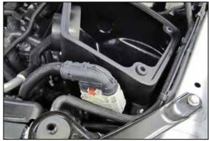
16. Clip the wiring harness onto the bracket installed onto the K&N® air filter housing.
