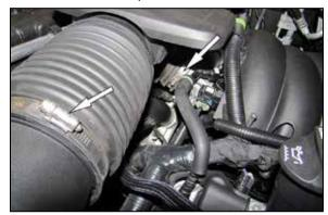
4. Loosen the hose clamps that secure the intake plenum assembly to the throttle body and air filter housing. Disconnect the plenum from the air filter housing and then rotate the plenum assembly counter clockwise to disengage the keyed mount and then remove the plenum from the throttle body.
