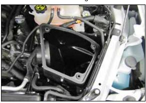
14. Install the K&N® air filter housing into the vehicle so the mounting grommets engage into the factory mounting holes. Secure the housing with the factory nut removed in step #9.
