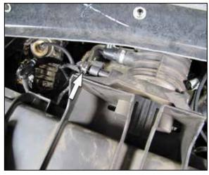
14. Pull the air filter assembly back slightly to expose "F" antenna at the top of the housing. Disconnect the electrical connection of the "F" antenna and then remove the air filter assembly from the vehicle. Remove the two fresh air duct extensions from the vehicle.
