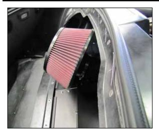
29. Push the intake tube towards the rear of the vehicle, install the filter onto the tube and secure with the provided hose clamp. Be sure to check the alignment before tightening the hose clamp, when the intake tube is installed the filter should sit horizontal.
