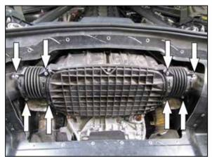
5. Remove the eight bolts that secure the two fresh air intake ducts and then remove the two ducts.
