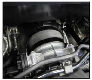
30. Insert the intake tube into the coupler at the throttle body and secure with the provided hose clamp. Be sure the tube and filter are aligned and straight before tightening the holes clamps.
