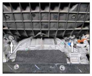
7. Remove the two bolts that secure the bottom of the air box.
