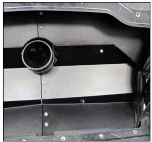
21. Peel the backing off the heat barrier and then apply the barrier to the engine side of the heat shield as shown. After the heat barrier is installed, use a knife or similar tool to cut out all of the mounting holes in the heat shield through the heat barrier.
