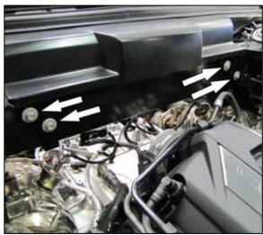
15. Install the two-heat shield mounting brackets to the chassis cross member using the four-air box mounting bolts.
