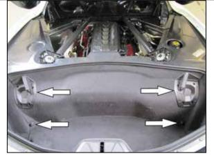
2. Open the rear hatch and locate the two roof stowage mounts. Remove the bolts that secure the stowage mounts and set the mounts aside. Remove the two wing nuts at the bottom of the compartment that secure the carpet.
