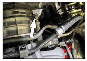
11. Cut the one time use clamp that secures the CCV hose and then disconnect the CCV hose from the factory intake tube. Loosen the hose clamp that secures the intake tube to the throttle body.
