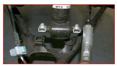
Remove the upper strut mount at the frame.
