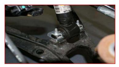
Install the sway bar end links and factory hardware. Do not tighten at this time.
