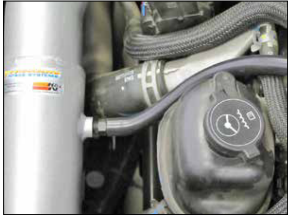
25. Reconnect the coupler to the valve cover port and then route the crank case hose to the fitting installed into the K&N intake tube and connect.
