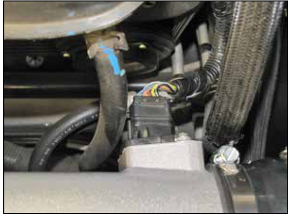
26. Reconnect the mass air sensor electrical connection.
