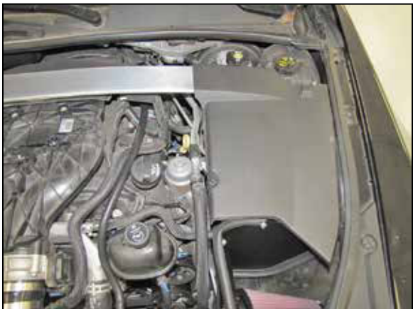
27. Reinstall the strut tower cover and snap it to the stand-off attached to the heat shield.
