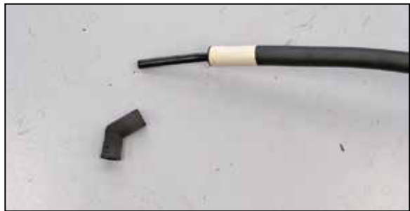
23. Remove the crank case vent tube coupler from the vent tube as shown.
