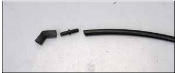
24. Install the union fitting into the coupler and then attach the provided crank case vent hose to the union.
