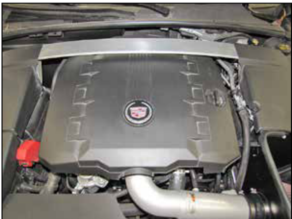
28. Reinstall the engine cover and oil fill cap.
