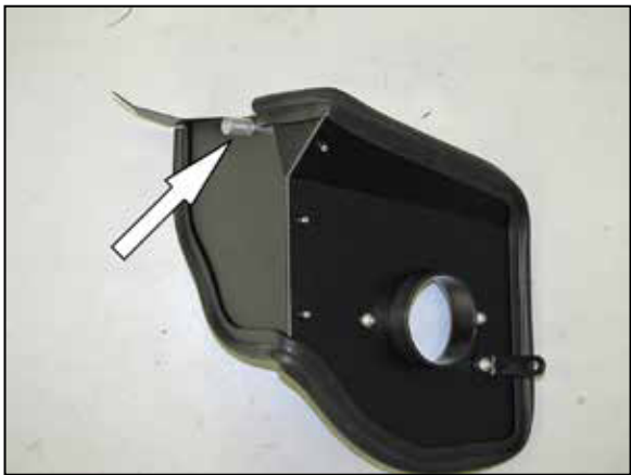
14. Install the 5/8"od aluminum stand-off onto the heat shield as shown.
