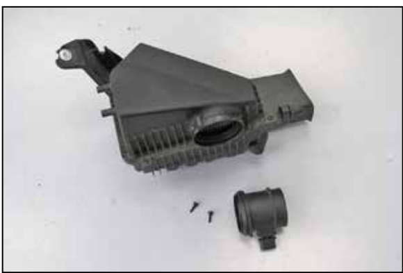
22. Remove the two bolts which secure the mass air sensor housing to the air filter housing and then remove the mass air housing. Remove the O-ring from the mass air sensor housing.
