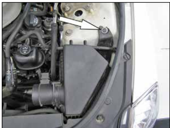
7. Remove the bolt securing the factory air filter housing into the engine compartment.
