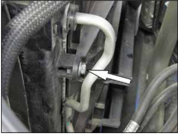
16. Remove the fan shroud mounting bolt shown. NOTE: This bolt will be reused in the next step.
