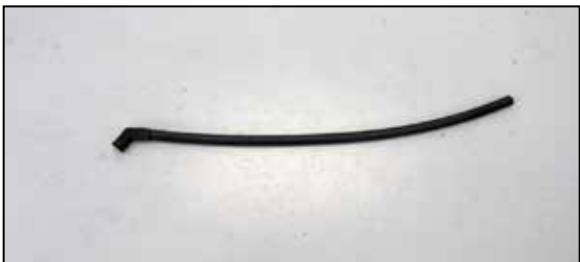
20. Attach the provided crank case vent hose to the hose mender as shown and then reattach the factory elbow to the valve cover.
