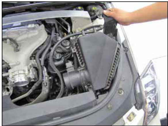
9. Remove the air filter housing from the vehicle. NOTE: The air filter housing has a forward facing mount out of view. NOTE: K&N Engineering, Inc., recommends that customers do not discard factory air intake.
