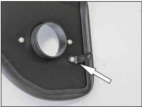
13. Install the "L" bracket (07805) onto the heat shield as shown.
