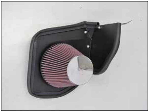
15. Install the K&N® air filter onto the filter adapter and secure with the provided hose clamp. NOTE: Drycharger® air filter wrap; part # RC-5107DK is available to purchase separately. To learn more about Drycharger® filter wraps or look up color availability please visit http://www.knfilters.com ®.
