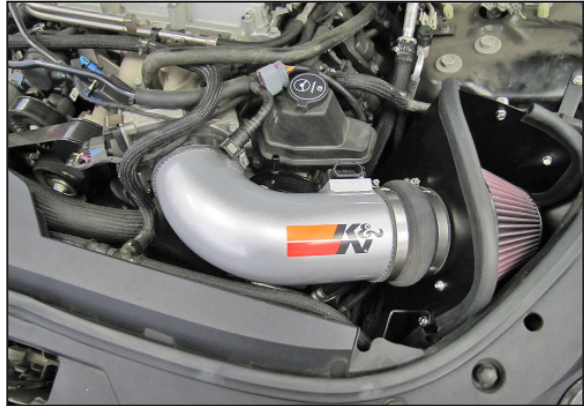
24. Install the intake tube into the coupling hose at the filter adapter and then into the hose at the throttle body, adjust the hose for best fit and then secure with the provided hose clamps.
