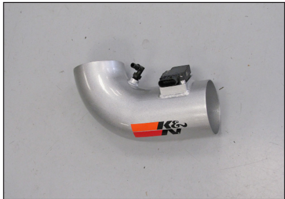
23. Install the 90° quick disconnect fitting into the K&N® intake tube as shown. NOTE: Plastic NPT fittings are easy to cross thread. Install the vent fitting “hand” tight, then turn it two complete turns with a wrench.
