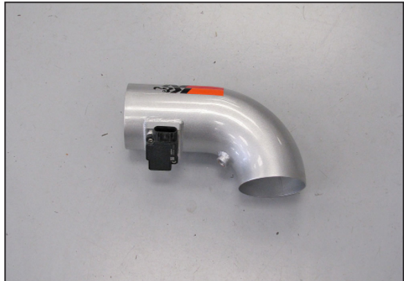
22. Install the mass air sensor into the K&N® intake tube and secure with the provided hardware.
