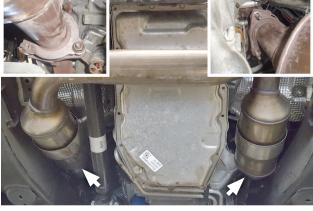
5. Remove (x3 ea.) nuts securing passenger and driver side exhaust manifolds to exhaust pipe. Then pull headers from their mounts.
