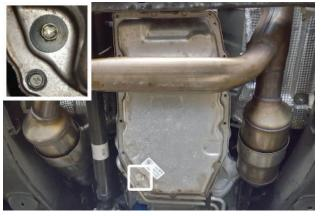
3. Place drain pan under transmission. Remove then wipe check bolt, while draining fluid from pan.
