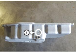
8. This kit includes a ½ NPT port above drain plug that can be used for an optional transmission temperature gauge. (available separately) Otherwise, install **NPT plug (8)**.
