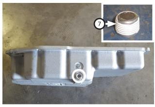
9. Apply Teflon tape to **socket plug (7)** before installing it into deep pan.
