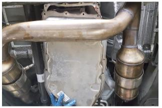
**NOTE:** Remove bolts starting from front of pan then moving laterally towards back to direct remaining fluid into drain pan.
