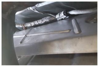
15. Allow exhaust to cool then re-install. Also install side cover and wire loom (removed step 4).
