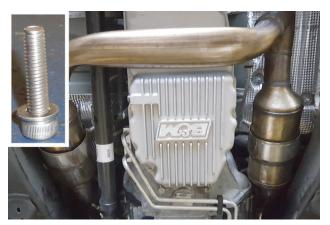
12. Use lint free rag to clean transmission pan mounting surface, then install deep pan with (x15 ea.) screws (2) and flat washers (3). Torque screws to 8 ft/lbs.
