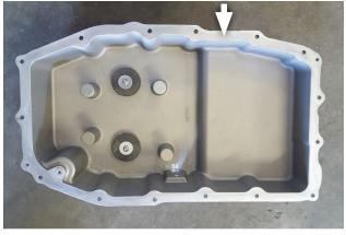
11. Inspect gasket (removed step 9) for flattened ridges or compressed edges then install it onto deep pan where indicated.
