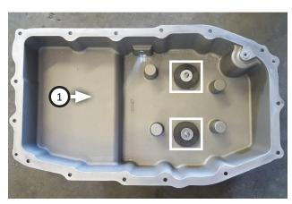
7. Install (x2) screws (5) through (x2 ea.) lock washers (4), flat washers (6), and magnetic rings (9) then into deep pan (1).
