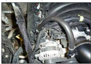
24. Connect the crank case vent hose assembly to the valve cover port and then to the fitting installed into the intake tube.
