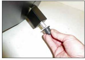
13. Install the provided grommet mount onto the heat shield using the provided hardware and then install the factory mounting grommet onto the mount as shown.
