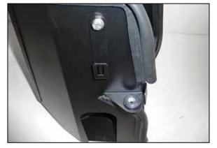
12. Install the provided wiring connector mounting bracket onto the heat shield using the provided hardware. Install the factory mounting grommet into the heat shield as shown.
