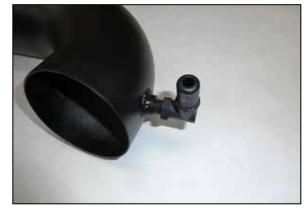
20. Install the provided 90° quick connect fitting into the  $K\&N^{\otimes}$  intake tube as shown.
