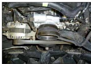
19. Install the provided reducer coupler onto the throttle body and secure with the provided hose clamp.
