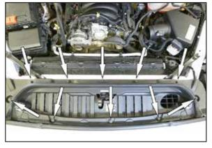
6. Release the ten retaining clips that secure the upper radiator valence and then remove the valence from the vehicle.
