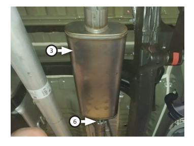
11. Route **tailpipe (4)** over axle then connect it to muffler. Insert wire hangers into isolators then tighten clamp just enough to allow for later adjustment.
