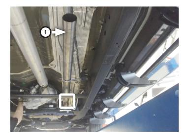
9. If applicable, place **clamp (6)** onto **extension (2)** then connect it to inlet pipe. Tighten clamp just enough to allow for adjustment.
