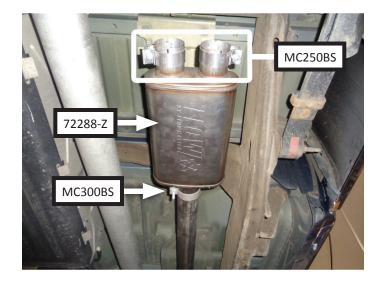
11. Locate following parts: bolt (HW209), left frame hanger (226HA), backing plates (x2) (HA566), flat washer (HW303), lock washer (HW309), nut (HW103). In following step, assemble parts as illustrated, with mounting surface located between backing plates.
