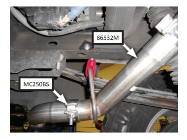
17. Place **2.5"** clamp (MC250BS) onto slip-fit of side exit pipe (86532M) then connect it to right tailpipe. Tighten clamp just enough to allow for adjustment.
