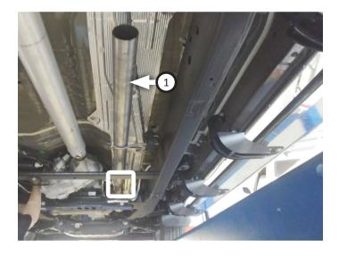
9. If applicable, place **clamp (12)** onto **extension (2)** then connect it to inlet pipe. Tighten clamp just enough to allow for adjustment.
