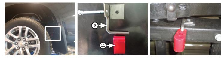
12. Route left front (4) and right front (5) tailpipes over axle then connect them to muffler. Insert their wire hangers into isolators and tighten clamps just to hold parts.
