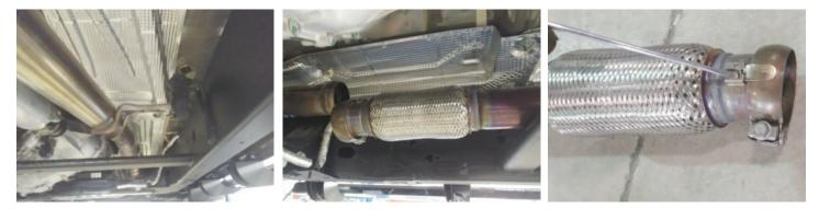
5. Remove nuts from stock and Flowmaster clamps, apply anti-seize compound to bolts and re-install nuts.
