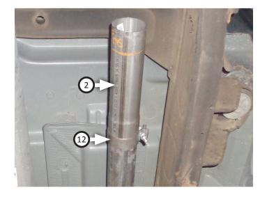
Place clamp (12) onto muffler (3) then connect it to inlet/extension pipe. Tighten clamp just enough to allow for adjustment then place (x2) clamps (13) onto muffler outlets.
