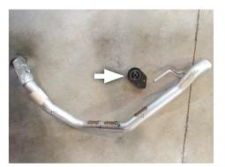
5. Cut tailpipes just behind factory muffler.
