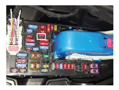
20. Connect female quick disconnect end of controller kit to fuse box.
