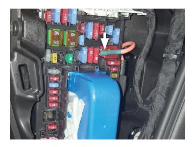
21. Connect ground wire of controller kit to metal frame under dashboard using **bolt (10)**, **flat washers (x2) (12)** and **nut (11)** as shown. Tuck any slack cord up and out of the way of vehicle operation.
