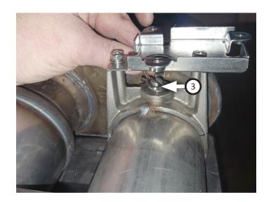
7. Place actuator motor (4) on actuator mount ensuring valve spring lines up properly. Secure parts using **bolt** assemblies (x3) (8).
