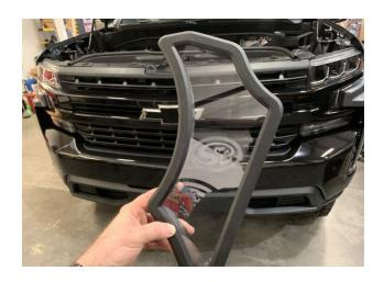
Install the Snap-In Lid Assembly into the S&B Airbox. The installation is significantly easier if the snap is slid into the curved section and its corners, first, then chase the snap around the profile of the lid, ending on the straight side.
