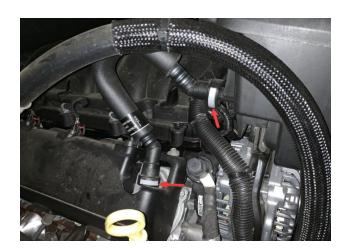
Loosen the hose clamp next to the MAF sensor and also the hose clamp on the throttle body.
