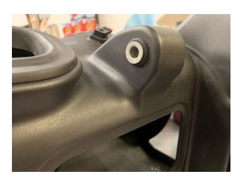
If desired, install the Silicone Box Plug (12) into the side of the airbox. The plug is designed to be able to be inserted from either the interior or exterior of the box; install according to preference
