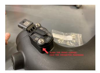
Screw the Quick Disconnect Adapter (11) into the Intake Tube (6).
