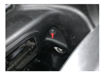
Insert the stock air inlet tube into the Inlet Seal on the S&B Air Box. The stop on the stock air inlet tube should be touching the seal when fully inserted. It may be helpful to guide the tube with one hand inside the airbox.
