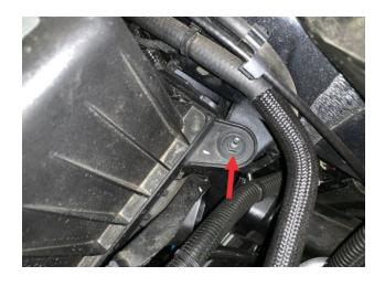
Remove the stock air box by lifting the front high enough to clear the stud, and pulling the airbox forward, sliding the rear-facing prongs out of the bracket
