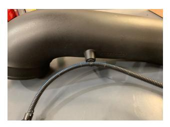
Install the intake tube into the vehicle, first mounting the coupler onto the throttle body, then swinging the tube down into the filter flange. Tighten all hose clamps.
