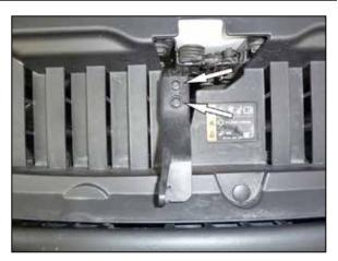
5. Remove the two bolts that secure the hood release arm to the hood latch and then remove the arm.
