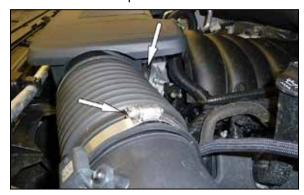
4. Loosen the hose clamps that secures the intake plenum to the air filter housing and to the throttle body. Disconnect the plenum connections at the air filter housing and then rotate the plenum counter clockwise to disengage the keyed mount and separate it from the throttle body.
