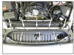
6. Release the ten retaining clips that secure the upper radiator valence and then remove the valence from the vehicle.
