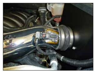
25. Connect the mass air sensor electrical connection.
