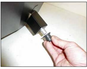
13. Install the provided grommet mount onto the heat shield using the provided hardware and then install the factory mounting grommet onto the mount as shown.
