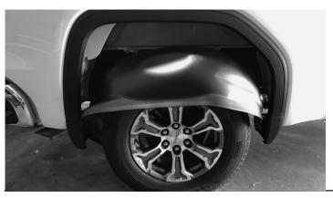
5. Insert the Wheel Well Guard into the rear wheel well opening over the tire.
