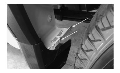
2. Reinstall 2 factory screws holding the factory rock guard on the front/rear side of the fender. These will need to be as loose as possible to allow the liner to slip between the mud guard and fender.
