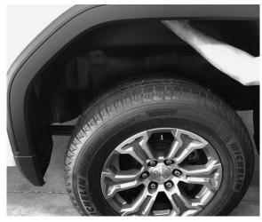
7. Push The Wheel Well Guard up into the wheel well opening. If the Wheel Well Guard acts caught and won't move upward check the 3 taps at B, C, and D locations. Shift liner forward to clear these areas.
