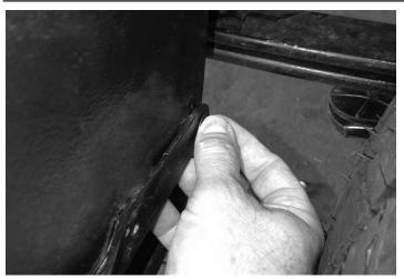
6. Tuck the Wheel Well Guard between the fender and factory mud guard. Start at the rear of the vehicle.
