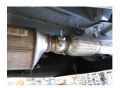
1) Place inlet pipe assembly #26409S into position onto the ball connection behind the catalytic converter. Reinstall the clamp onto the ball connection and tighten enough to hold, but still allow for a small amount of adjustment. Connect the hanger on the pipe to the rubber mount on the vehicle.
