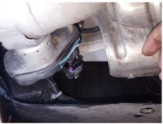
3) Behind each rear tire, remove screws (x2 ea.) attaching lower cover to frame. Unplug electrical connection from actuators then dismount both front wire hangers on muffler from rubber isolators.
