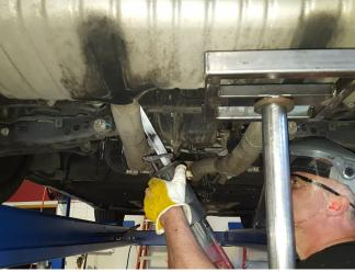
2) Begin by measuring back 1-½" from rear of suspension cross-member (as shown) and make a mark on both pipes. Support exhaust system; both in front and behind area to be cut. Once you've double checked measurements, cut both pipes at their marks. **Note: Use caution when cutting!**
