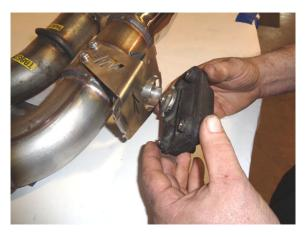
1) Remove bolts (x3) securing exhaust actuators to factory muffler assembly. Place them onto mounts on new Flowmaster units then fasten them by re-using bolts (x3).
