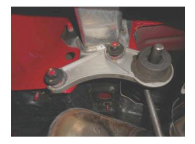
Carefully deburr factory pipes at cut ends. Remove hanger mounts at rear of vehicle from vehicle frame and transfer them from factory system to corresponding side on Flowmaster system.
