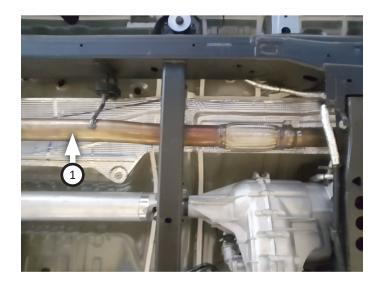
8. If applicable, place **clamp (14)** onto **extension (2)** then connect it to inlet pipe. Tighten clamp just enough to allow for adjustment.
