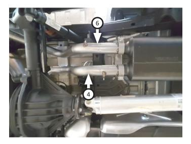
12. Place clamp (13) onto left rear tailpipe (5) then connect it to left front tailpipe. Insert wire hanger into rubber hanger then tighten clamp just enough to allow for later adjustment.
