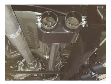
11. Fasten frame hanger (10) to vehicle frame (behind rear driver tire) with bolt (14), (x2) backing plates (11), flat washer (15), lock washer (16) and nut (17). Then fit rubber hanger (12) onto frame hanger.
