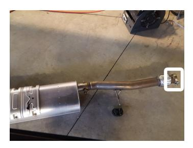
11. Remove nuts from stock and Flowmaster clamps, apply anti-seize compound to bolts and re-install nuts.
