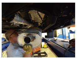
10. Release tab and remove clamp from muffler assembly. Retain for later use.
