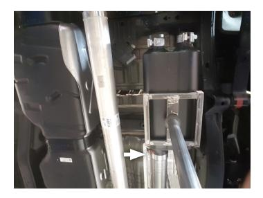
15. Route **right (4)** and **left (5) front tailpipes** over axle and connect them to muffler outlets. Mount wire hangers in isolators then tighten clamps (x2) enough to hold parts.
