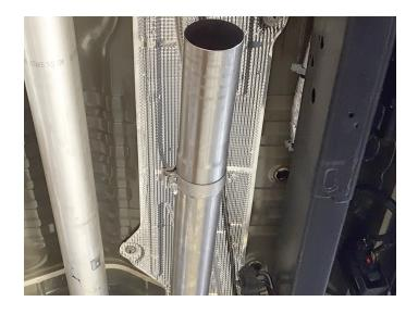
14. Place clamp (8) onto muffler (3) inlet. Place (x2) clamps (9) onto muffler outlets. Connect muffler to inlet or extension pipe then tighten front clamp just enough to allow for adjustment.
