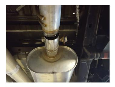
8. Disassemble tailpipe wire hangers from rear isolators then remove remaining tailpipe from vehicle. Retain isolater and bolt for later use.
